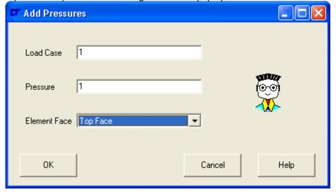
Choose the Top Face of the element, put in a value of 1 for the pressure and press the OK button.
