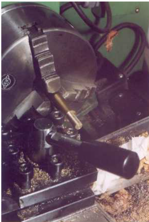
Machining the Pivot Bolt from 1/2" brass bar:-
