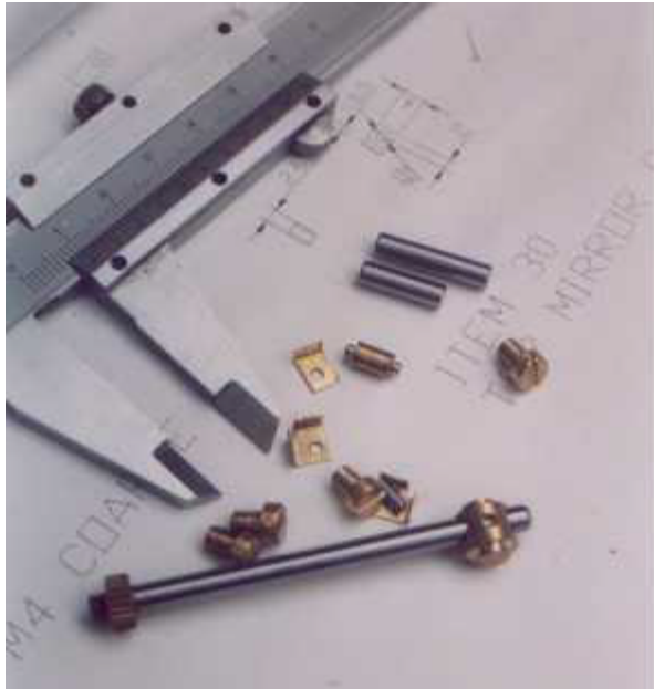
Machining the Pivot Bolt from 1/2" brass bar:-
